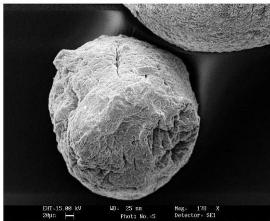
**Figure- 5: SEM photographs of Pioglitazone hydrochloride microcapsules**
