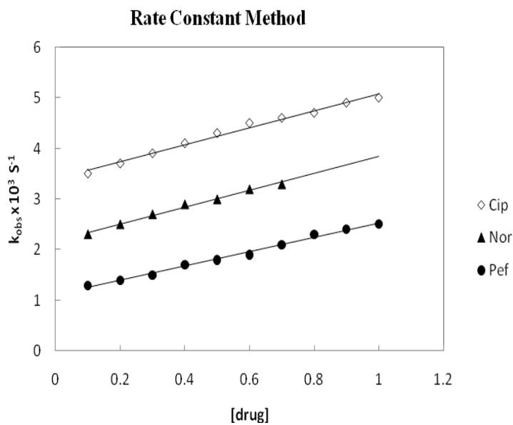
Figure 2: Calibration graph of Fluoroquinolones for Rate constant method
