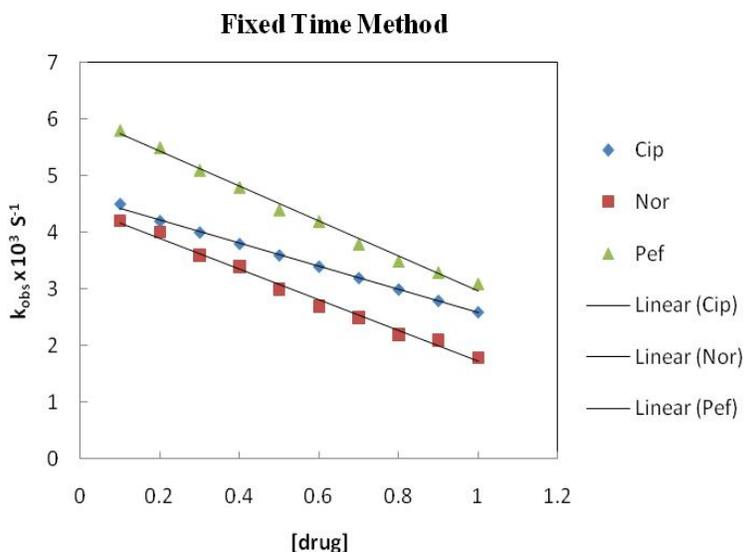
**Figure 3: Calibration graph of Fluoroquinolones for Fixed time method**
