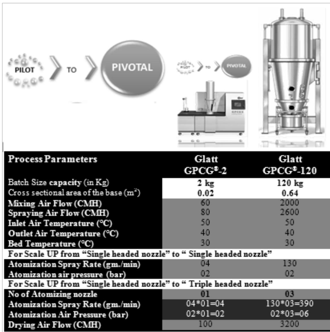
**Figure 5.** FBP Parameters from small scale to large scale
