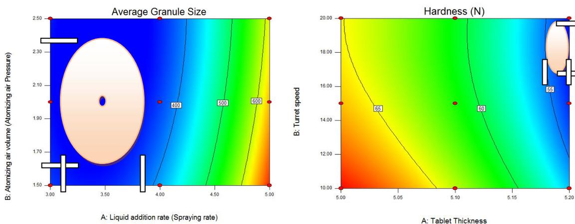
**Figure 3:** Design Space & Edge of Failure: (a) for FBP (b) for Compression
